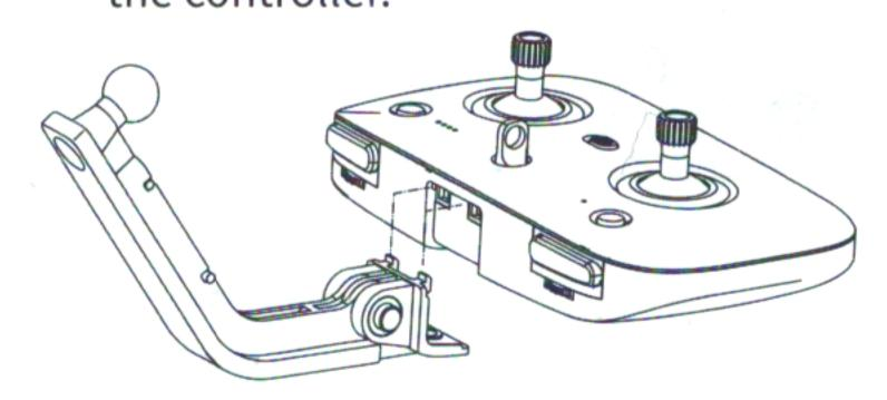
2 Insert and tighten mounting bracket screw (M5\*8).
