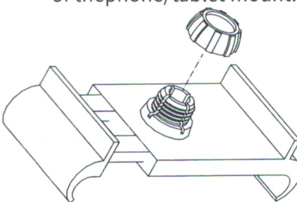
4 Place nut over mounting bracket swivel ball. Then snap mounting bracket onto phone/table mount and tighten nut.
