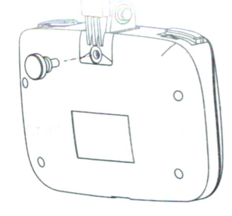
3 Remove the nut on the back of thephone/tablet mount.
